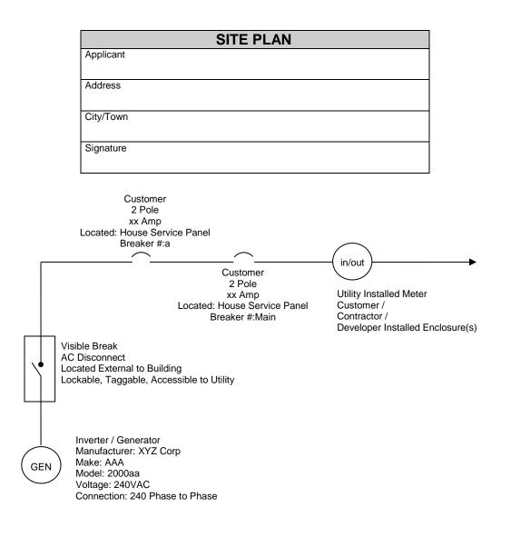
Note: This One-Line Drawing is a general drawing for Net Metering customer. Legible hand drawn one-line drawings are acceptable.
